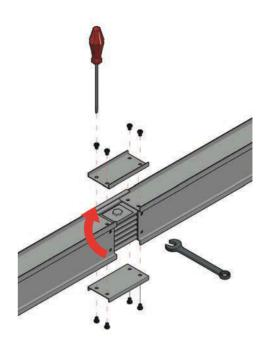
Install the additional block to the busbar and fix it to the next length body.
