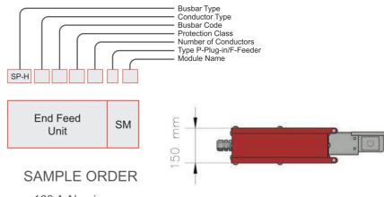
160 A Aluminum, Feed Unit IP 55 5 Conductors
